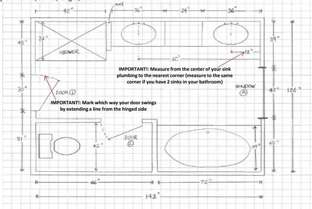
Measure carefully and double check all measurements. Measure from outside of casing to outside of case. Mark direction of door swing(s) on provided floor plan grid.
